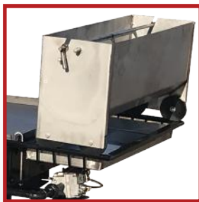
Batter dispenser sitting over the drip pan area
